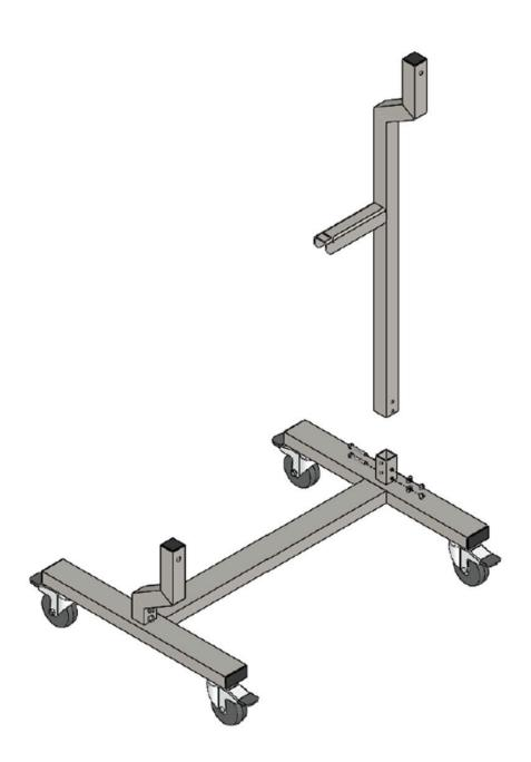
5. Slide 2 x through support bars through the conveyor body. Then, slide 2 x through stops onto the protruding ends of the through support bars. Ensure the lip on the through stops is flush with the sheet metal. With the through stops installed, and with the help of another person, slide the protruding bars into the short H-base upright and tall H-base upright and fasten with 2 x 1" button head screws.
