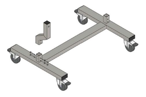
4. Install the TALL H-BASE UPRIGHT to the H-BASE using the same hardware in the last step.
