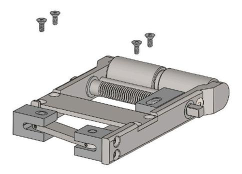
6. Using a 5/32 hex key, remove the 4 screws securing the plate to the two side arms.
