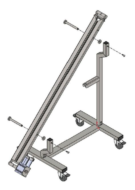
Install the belt onto the conveyor body by simply sliding it onto each end.
