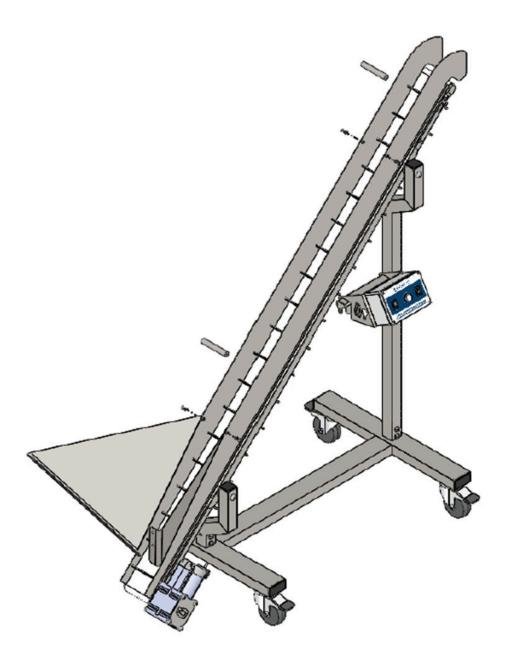
Finally, to complete the hopper assembly, install the BACK PLATE on to the outside of the side panels by aligning the screw holes and securing with 6 x <sup>3</sup>/<sub>8</sub>" BUTTON HEAD SCREWS. The screw heads should go on the inside of the hopper, and the 6 x ACORN NUTS can be used on the outside to firmly secure the BACK PLATE.
