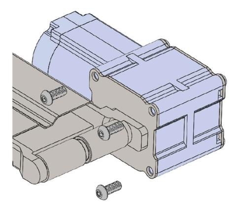
3. Using a 9/64 hex key, remove the 4 bolts securing the motor assembly to the conveyor body. Removie the motor and set these aside in a safe place.
