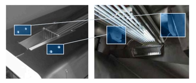
3. The Adjustment Blocks are fastened to the interior of the body during shipping. To install, they will need to be removed using a 5/16 hex bit or Allen Key to loosen off the bolts on the exterior of the body. Place the Adjustment blocks over their corresponding holes on the exterior of the body and fasten them from the interior of the body using the same bolts and 5/16 hex bit or Allen Key. Insert hopper Pins into Adjustment Blocks to lock hopper in position.
