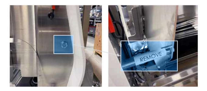
4. If the supports aren't removed, the operator will not be able to disassemble the belts off for cleaning.
