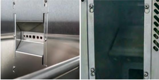
To get started, position the MBX in your work area, lock the casters and check that the front die plate and rear guard window are secured in place.
