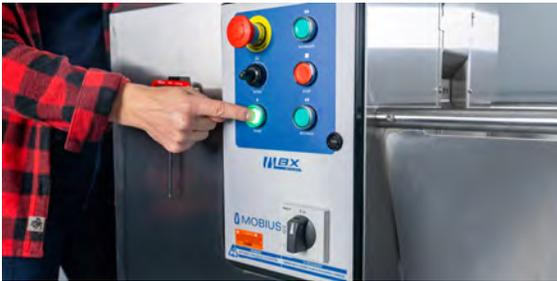
If the e-stop is engaged, release it and press the START button to fire up the chipper.
