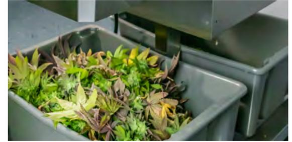
Place a tote under the front of the machine to collect the flowers and leaves and a second tote under the back of the machine to collect the chipped stalks.
