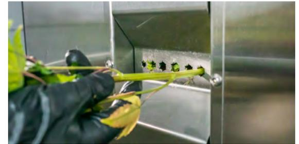
Begin feeding the bottom end of your stalks into the holes in the die plate, trying to match the stalk with the smallest diameter hole that it will fit into.
