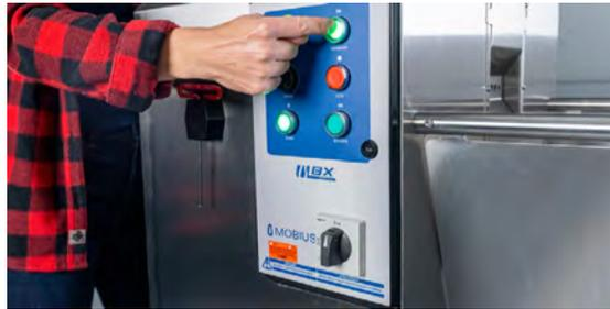
Press the FORWARD button to start the rolls and rotate the speed dial to your desired setting.
