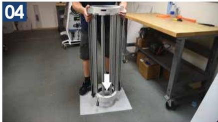
Put some padding on the floor. Stand the lid on end. Lift the lid a few inches off the floor and bring it back down squarely on the pad. You may have to do this a few times to create a gap between the black ring and the white Edna.
