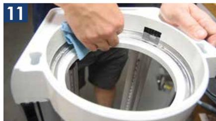
You may find soiled grease, plant material, or bits of O-Ring cord inside the Edna. Use a degreaser and a rag to clean it.
