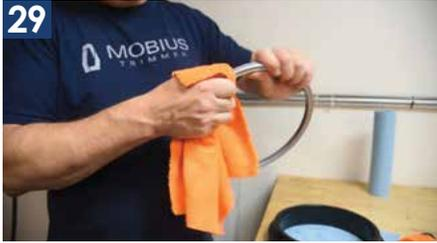
29 With the bearing removed, assess its condition and clean or replace as necessary.
