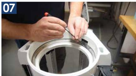
With the black ring removed, set the lid on end again but with the end you're working on facing up. Use a pick to gently lift the O-Ring cord out of its seat
