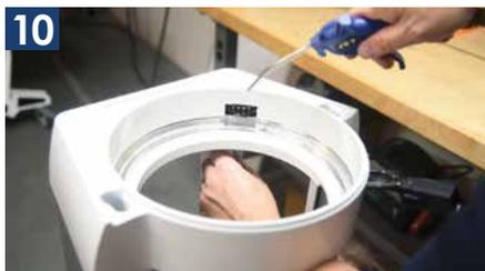
You may need to use a pick, a degreaser and compressed air to clean each tooth of the drive cog. Once cleaned, swing the hex bar back out of the way and gently tighten the bolts
