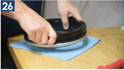
26 Place a cloth on a solid work surface. Squarely bump the black ring down on the surface to cause the bearing to slide down the hub of the black ring. Use this method until the bearing touches the table top
