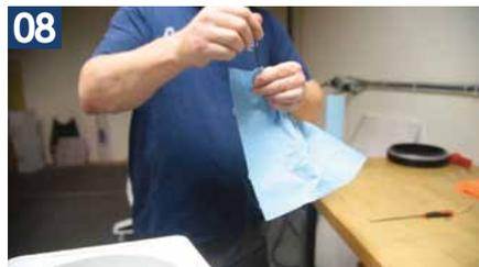
Gently wipe the O-Ring clean of grease and debris using a clean rag. Be careful not to stretch the O-Ring cord as you're pulling it through the rag
