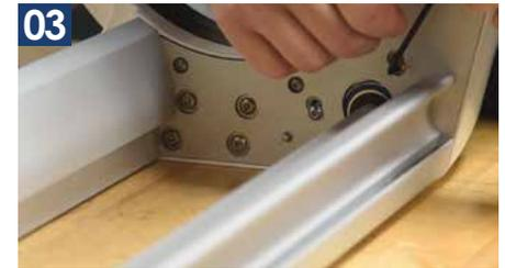
Loosen the bolts far enough to slide the hex bar away, disengaging the hex bar drive from the black ring
