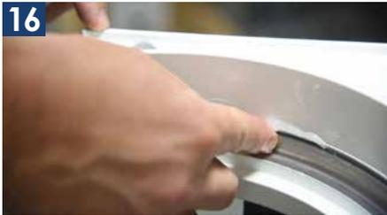
16 Add a good bead of SuperLube to the leading edge of the O-ring to assist in pressing the black ring back into the Edna.
