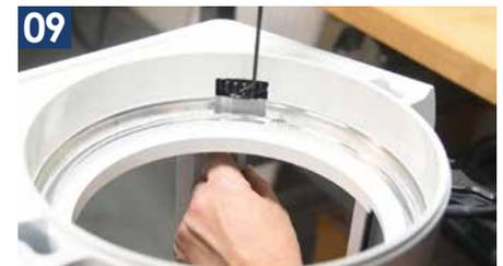
Loosen the hex bar bolts a bit and move the hex bar drive into the access window where it can be cleaned.
