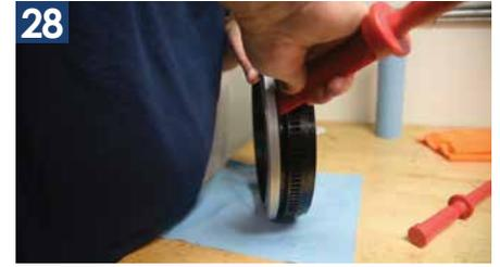
28 Use a soft pry, and pry only the inner race to remove the bearing from the black ring
