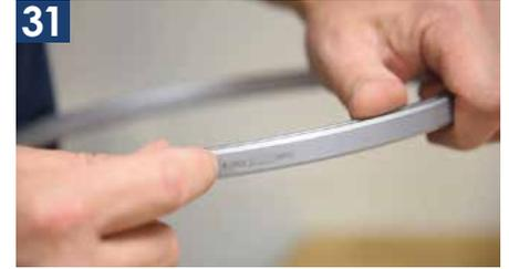
31 To install the bearing, find the directional arrow and install in that direction.
