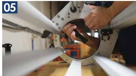
Place the lid back on your work surface. Using a plastic pry, widen the gap uniformly, being careful not to cock the black ring diagonally within the Edna. If using a metal pry bar, use a piece of cloth between the components and pry bar. Be careful not to dig into the black ring or the Edna with your pry.
