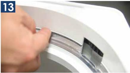
13 Make sure the O-ring cord doesn't protrude into the drive gear window.
