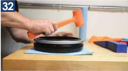
32 Gently and evenly tap the bearing into place using a soft mallet and a block of plastic, brass or wood to fully seat the bearing on the black ring
