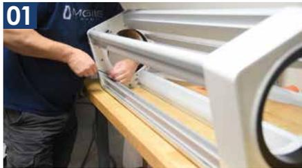
Remove the lid and set it on a stable work surface. Using a 1/8" Allen Key, loosen the bolts holding the hex bar in place.
