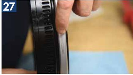
27 These bearings are directional. Force must not be applied to the outer race against the direction of the arrow printed on the side of the bearing race.
