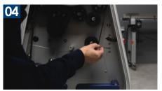
Remove the 1st and 3rd screws here as well.
