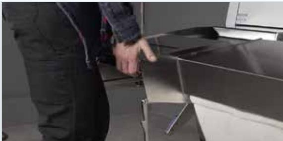
Because the separator is not fully installed, there is no support coming from the fan housing yet, which can cause the separator to tilt to one side. If you've ever found it challenging to install your separator, this is why.
