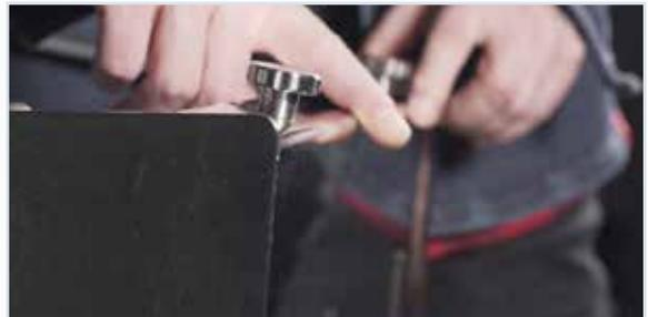
Installing the facia in a way that leaves an air gap around the window will result in reduced vacuum and compromised trim quality.
