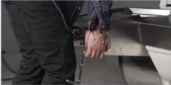
With the top side of the separator approximately parallel with the floor, begin sliding the separator into place, recognizing that the guide rail on the left side of the separator will be sliding on top of the support rail on the body of the machine.
