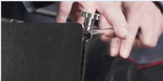
The top section is then secured into place with two tension knobs. It is vitally important that the facia and window form a tight fit with the separator body. Once assembled, the separator must be air tight so that maximum vacuum and trim quality can be achieved.
