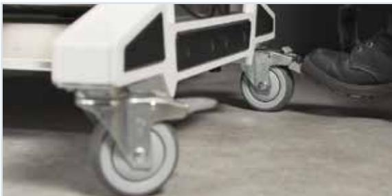
Ensure that at least two of the casters are locked so that the trimmer does not move as you are installing the separator.
