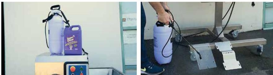
Using a mixture of SuperClean and hot water, spray both these components and let them sit.
