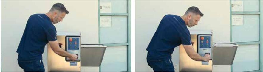
First, push the e-stop button, rotate the lockout to the off position, and unplug the machine.
