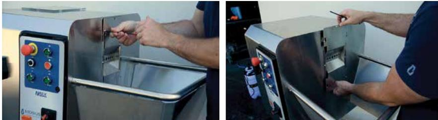
Remove the stem hole dieplate from the front of the machine by unscrewing the 4 screws at the corners, then sliding the plate up and off.
