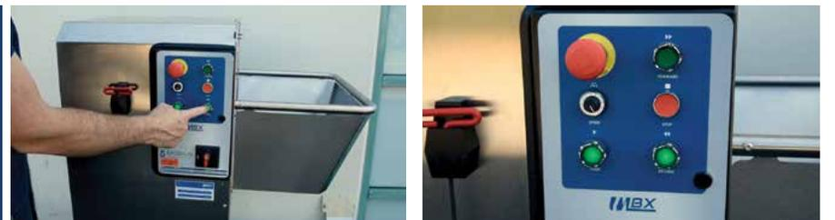
Plug the machine in, disengage the lockout and turn it on, making sure to select 'reverse direction'
