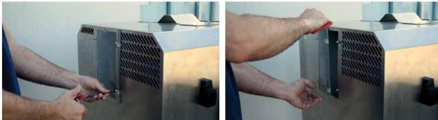
Remove the plexi panel covering the stem chipper on the back side of the machine in the same way.
