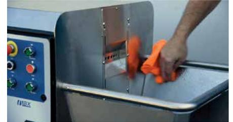
Reinstall the covers. Wipe down the whole machine to remove any remaining water.
