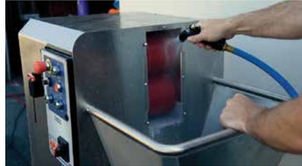
Remove the dieplate covering the rollers and rinse with water
