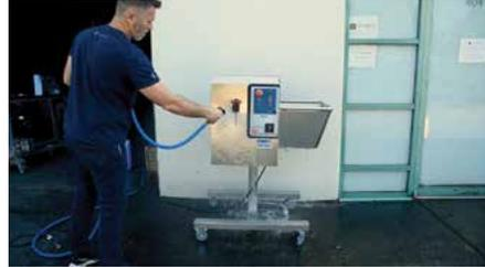
Turn the machine off, unplug it, and rinse it with water.
