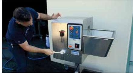
Allow the rollers and chipper to spin while the rest of the machine is sprayed with the cleaner to remove any plant debris and residue. You can use a soft brush to clean off any plant material that is more difficult to remove
