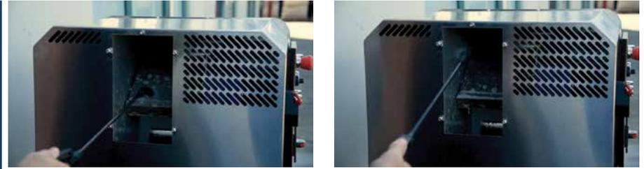
Spray the chipper, rotating it to spritz all sides with cleaner, and continue spraying the interior surfaces.
