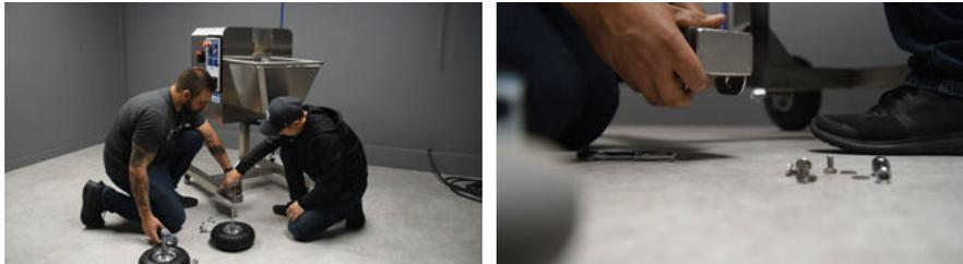
Place one of the u-shaped brackets over the foot of the bucket, aligning it approximately with where the old wheel was.
