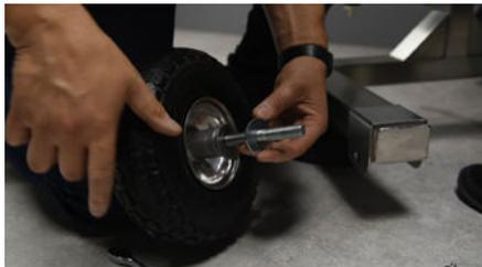
Remove the nut and one of the large washers from the end of the axle on one of the outdoor wheel assemblies, keeping the rest of the assembly intact.
