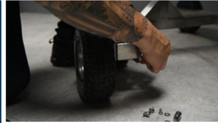
Place the washer and the nut on the end of the axle.
