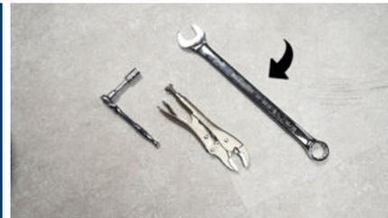
Using a 15/16" box end wrench or socket, tighten the nut. Repeat these steps for the 3 other wheels.
