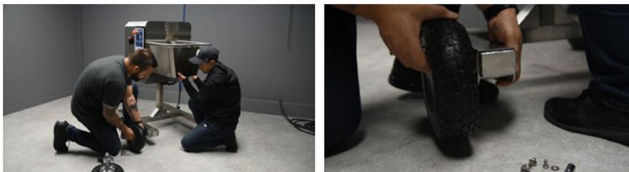
Align and push the axle of the wheel assembly through the hole in the bracket
