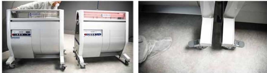
To prevent interference, position the unit wheels so they're pointed back towards the body.
