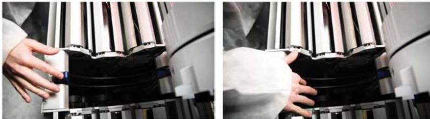
Rotate the tandem locks inward until the handles are pointed down.
