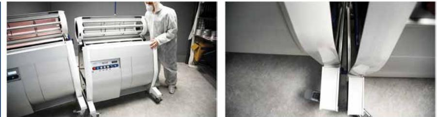
Move infeed unit and align as closely as possible.
