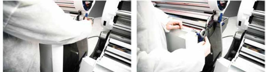
Place tandem locks on the outfeed unit conveyor sensors, pointed up.
