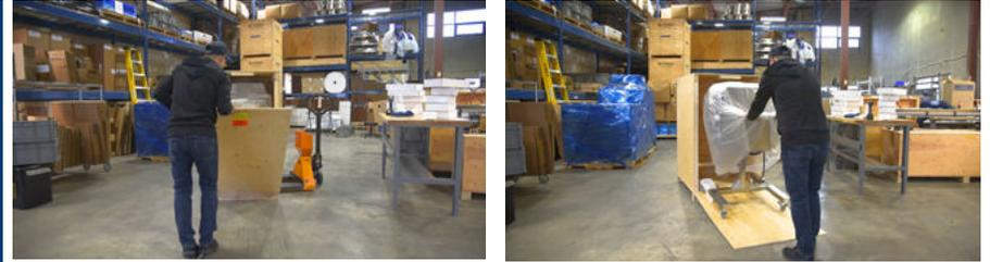
Use the wood panel you removed to act as a ramp to roll the bucker out of the crate.
