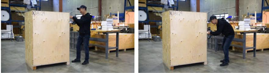
Remove the screws on the side of the crate with the 'Open This End' label.
