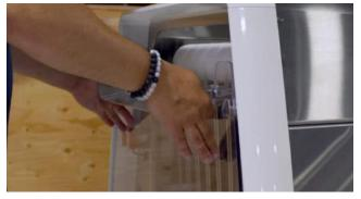
Install the inlet cover on the infeed side of the machine and the outlet cover on the outfeed side of the machine, ensuring that the bands are positioned between the metal grooves on the outlet cover.
