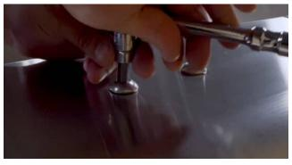
Next, we'll get the feed area sorted. The blocks for the feed hopper are mounted inside the machine for shipping, so begin by removing these four bolts with your hex wrench and mounting the blocks on the top side of the machine, channels facing inwards.
