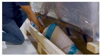
Before we move the machine off the crate base, set aside all of the loose parts: some of these parts are resting on the crate base under the machine and some are packed inside the machine. Video instructions are available online for your reference.
