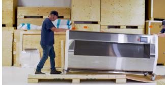
The Mobius M9 is a sizable machine; set yourself up in an area with enough clearance to access all sides of the crate. Once the crate top and side panels are removed, the machine will be rolled off the end of the crate base; it's vital to leave enough space at one end to accommodate this.
