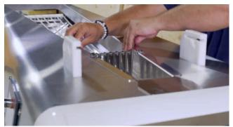
The inlet guide can now be installed.
