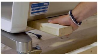
Using the 2-by-4 that spans the crate between the machine base and unibody as a lever, have the two people on either side lift the machine up a few inches; the third person can now slide out the wooden block.
