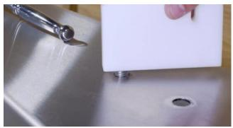
Now reverse the feed hopper blocks and screws and tighten the bolts to the blocks from underneath.
