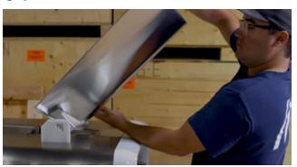
Once you have both feed hopper blocks installed properly, install the hopper into the blocks.
