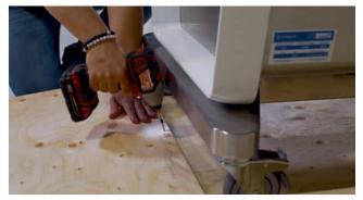
Use one of the end panels from the crate as a ramp so that the machine can be rolled off the crate base. Using the lip of the crate base for support, place an end panel down as a ramp and secure it into place with a wood screw.
