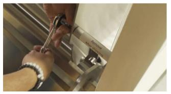
Remove the shipping standoffs; they exist to give the body rigidity during transport. Open the back cover of the machine and locate the two standoffs labeled "Remove after shipping". Using a 5/16ths hex wrench, unscrew the bolts on the standoffs and set these pieces aside. They are not needed for normal assembly and operation of the M9 and can be disposed of after this step.
