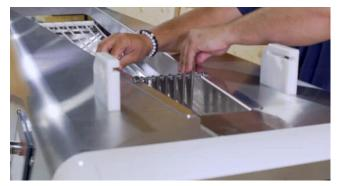
The inlet guide can now be installed.
