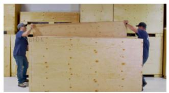
Now, remove the screws along the bottom of each long side panel and set these panels aside. Finally, remove the screws holding the end panels in place and set these panels aside. Disassemble the crate.
