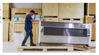
The Mobius M9 is a sizable machine; set yourself up in an area with enough clearance to access all sides of the crate. Once the crate top and side panels are removed, the machine will be rolled off the end of the crate base; it's vital to leave enough space at one end to accommodate this.
