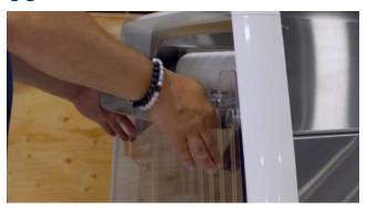
Install the inlet cover on the infeed side of the machine and the outlet cover on the outfeed side of the machine, ensuring that the bands are positioned between the metal grooves on the outlet cover.
