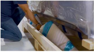
Before we move the machine off the crate base, set aside all of the loose parts: some of these parts are resting on the crate base under the machine and some are packed inside the machine.
