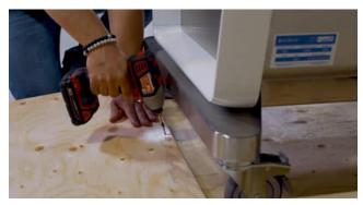
Use one of the end panels from the crate as a ramp so that the machine can be rolled off the crate base. Using the lip of the crate base for support, place an end panel down as a ramp and secure it into place with a wood screw.
