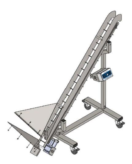
10. Using the TENSIONING TOOL, turn the BELT TENSIONING STUB to ensure that the belt is properly tensioned. DO NOT OVER TORQUE THE BELT TENSIONING STUB, PERMANENT DAMAGE MAY RESULT. The TENSIONING TOOL can be stored in the keyhole cutout on the CONTROL BOX.
