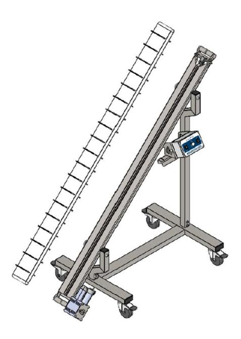
7. Install a SIDE PANEL on each side of the conveyor by aligning the circular cutouts with the THROUGH STOPS and THROUGH BARS. Simply slide each panel down onto the pucks to install it on the conveyor.
