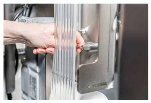
Move to the back side of the Sorter and open the tailgate by releasing the two 5 compression latches.
