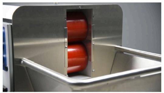
2. Remove the front dieplate to expose the rolls.
