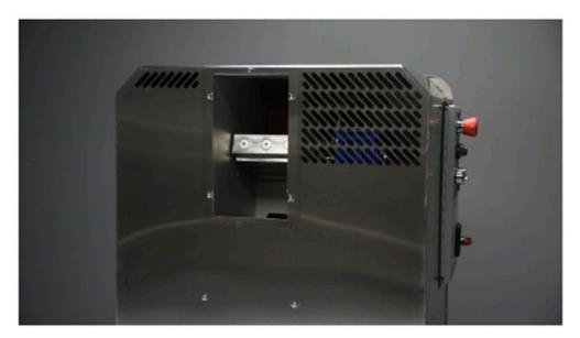
4. Using hot water, spray or pressure wash the interior of the machine. Use caution not to pressure wash the rolls directly, as the high-pressure jet may damage the rolls.
