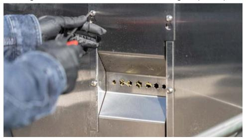
3. Remove the rear guard window covering the stem chipper on the back side of the machine in the same way.
