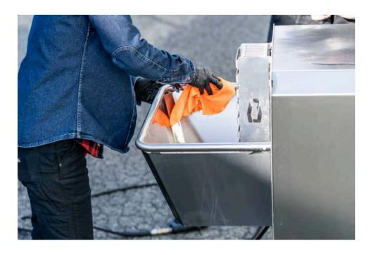
11. Once you're done with cleaning, unplug the machine and remove the cleaning plates. If desired, all components can be sanitized with Shyield or ISO. Reinstall the front bucking die plate and rear guard window.
