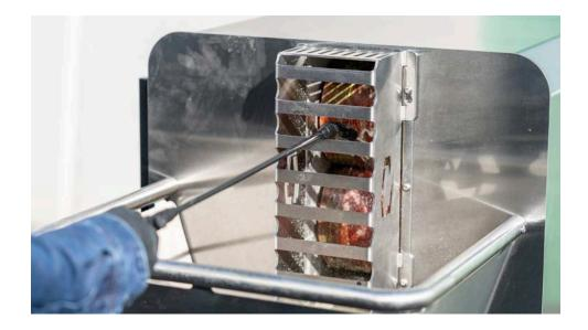
**NOTE:** The electrical panel and rear of the Bucker should never be hosed or sprayed directly. Use caution not to spray near the motors or into the vents in the rear of the Bucker.
