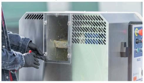
4. Swap your front bucking plate and your rear guard window for the MBX cleaning plates. Once the cleaning die plates are secured, the machine can be plugged back in to start the cleaning process.
