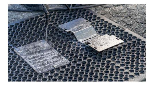
8. Use a hose or a pressure washer to spray through the front and rear dieplates to clean off the rolls and chipper. If the resin build up is heavy, you may need to apply a second round of cleaner and rinse again. You can also use a long handled brush to help remove resin build up on the rolls. Use caution not to pressure wash the rolls directly as the high-pressure jet may damage the rolls. Use hot water to improve the efficacy of the cleaning solution.
