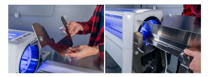
To pair the Mobius Outfeed Conveyor to the M108S Trimmer, simply roll the conveyor into place, either inline with the trimmer or at a right angle, in either direction.
