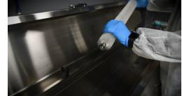
Remove the brush by grasping it at both ends and pulling gently to release it from the clips. Rinse off and set aside to dry. We recommend using the end bearings as support during drying so that the bristles do not dry flat.
