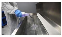
Begin by filling washer basin approximately half full with warm or hot water. The fill slots on the motor mount plate will prevent you from over-filling the basin. It is recommended that water temperature not exceed 65°C (150°F).
