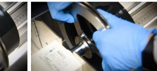
Lift the left end cap and slide it towards the motor to align the drive cone. Rotate the assembly to align the drive pin with one of the holes in the spreader plate. As you do so, the shaft at the knob side should fall down into place on the plastic support.
