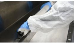
Lift the spreader at each end and lower it into the basin, resting the knob-end on the plastic support on the right-hand side.
