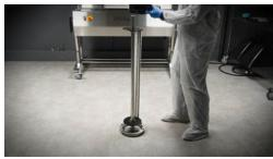
Remove the spreader assembly from the washer and place the drive (left) end on the ground
