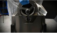
Remove the spreader from the basin by lifting the right hand side and sliding to the right to disengage drive pin before lifting the assembly fully out of the basin. Set the assembly down and rinse off. Remove tumbler from spreader.
