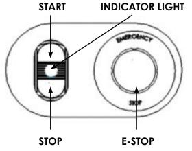
**E-STOP** - Prevents accidental start-up, used for servicing and removing components.
