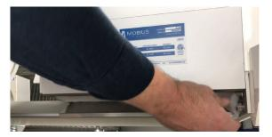
Tuck the loose (right) end of the filter mesh into the corner above the bolts. INSIDE VIEW
