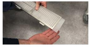
The left side of the filter holder and filter mesh should be flush, while the right side will have a small strip sticking out.
