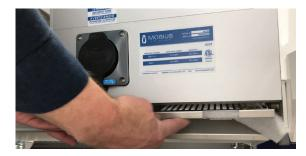
Ensure the machine is unplugged. Orient the filter holder with the metal grate facing up and the filter just below it. Push the filter assembly into place by hooking the lip on the lower side of filter holder onto the base of the trimmer. No tools are necessary - the assembly will slide into place.
