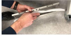
Start by tucking the filter mesh strip into the filter holder. Work your way around the edges until the filter mesh is seated flat against the grate of the filter holder.
