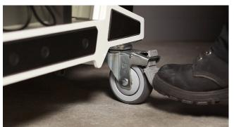
Lock the machine into place and open the lid.
