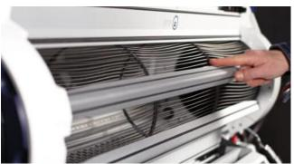
Before tensioning the tumbler, it's important to check the alignment of the wires. Working from one end, trace one of the tumbler wires across to the other end. Rotate the loose end as necessary to ensure that the tumbler wires will be straight once under tension. Video instructions are available online for your reference.
