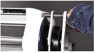
Next, grab your Spring Jack tool and position the two handles and the valve in the middle vertically, with the knobs on the back pointed down.
