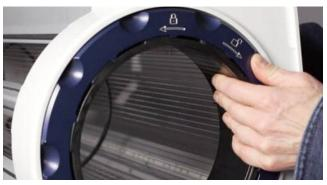
Give the tumbler a quick back and forth rotation to ensure that it moves freely.
