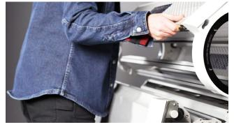
The lid should always be open when the tumbler is not under tension, so that the wires are not caught on the blade components.
