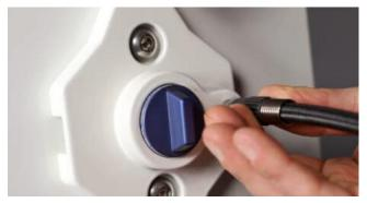
Attach your air supply to the Schrader valve on the Spring Jack and apply enough pressure to bottom out the spring pack in the lid. This will typically run between 100 and 130 PSI. The number itself doesn't matter; the purpose is to give ourselves enough slack on the tumbler to get the opposite retaining ring on.
