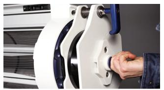
Rotate and lock the air valve into place. The handles and valve dial will now all be in one line.
