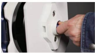
The final and most satisfying step can now be taken! Push in and rotate the valve dial on the Spring Jack counterclockwise.
