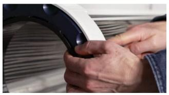
To install the retaining ring on the opposite side of the tumbler, position this one with the ring tabs alternating with the tumbler end cap tabs, as with the first retaining ring. Position your hands so that your fingers are pulling out on the black tumbler end cap and your thumbs are pushing in and rotating the blue ring into the locked position. Again, no silver on the ring tabs should be visible.
