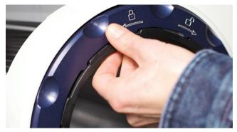
Once the tumbler is loosely positioned within the lid, install one of the blue retaining rings onto the infeed end. The tabs on the ring will show silver and alternate with the tabs on the tumbler end cap when unlocked.
