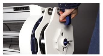
Insert the Spring Jack into the receiving holes on the lid and rotate the handles inwards.
