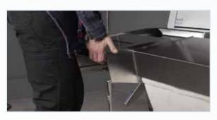
Because the separator is not fully installed, there is no support coming from the fan housing yet, which can cause the separator to tilt to one side. If you've ever found it challenging to install your separator, this is why.
