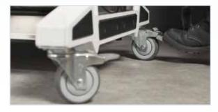
Ensure that at least two of the casters are locked so that the trimmer does not move as you are installing the separator.
