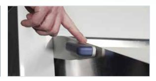
The top edge of the hockey stick will be parallel with the top side of the separator. That's all there is to it!
