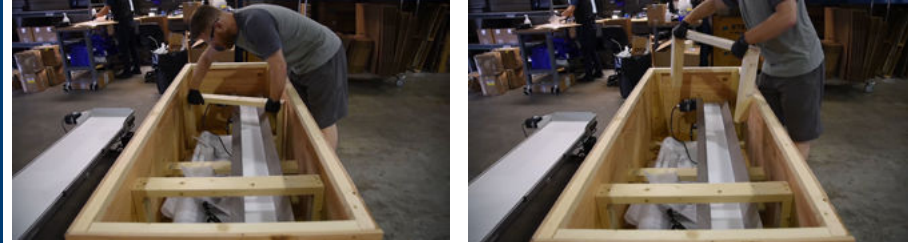
Remove the bridge using a slight bump to knock loose and lift out.
