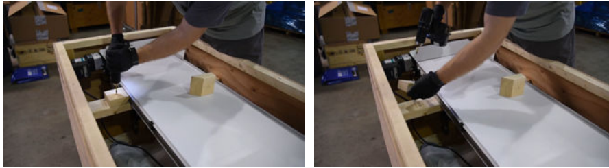
Unscrew custom wooden wedge bracing the sides of the conveyor.
