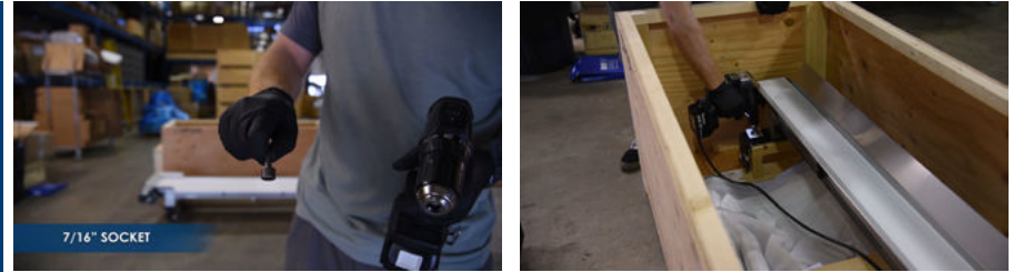
Using a 7/16" nut driver or socket, remove the bolts, washers and vinyl strip that secure the infeed conveyor to the saddles.
