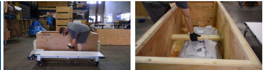
Unscrew the single 2x4 in the centre from the outside securing the legs.
