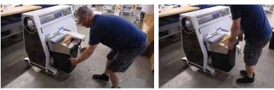
Swivel the latches towards you slightly and up so that it raises the Trim Tote and seals off the gasket, locking it in place.
