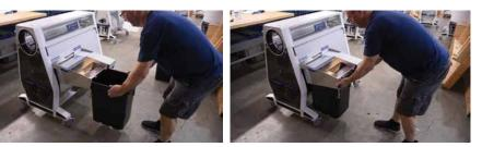
To install the Trim Tote, slide it on the rails of the separator with the warning symbol going in first.
