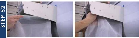
Slide the retaining ring up into the housing past the rail and allow it to fall into place. Give it a slight tug to make sure it's seated properly.
