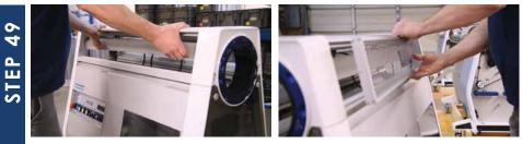
Install the brush bar by pushing it into the receptacles on either side of the lid. Both sides of the brush bar are identical so it can be installed in either orientation. Re-install the front screen
