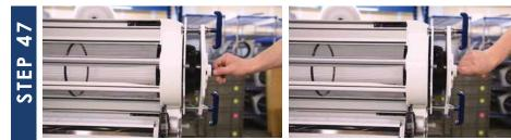
Now, on the Spring Jack, turn the air-release valve to the open position. This will release the air to apply tension to the tumbler. You'll see the cables of the tumbler pull tight.
