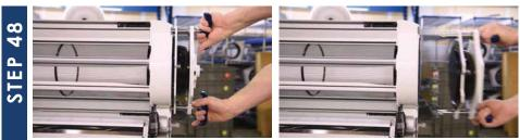
Rotate the handles of the Spring Jack outwards to release from the lid. Make sure the tumbler rings are in the locked position, the tumbler is under tension, and can rotate freely. Now, close the lid.
