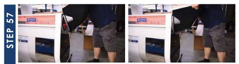
Install the hopper on the infeed side in the same way as the chute, its opening facing up. Hook the lip into the ledge on the lid and rotate the base into place. The red light will turn blue when all errors are cleared, indicating the machine is ready to run.
