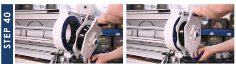
Unpack the Spring Jack Tool, and insert the handlebars into the receptacles on the infeed side of the lid.
