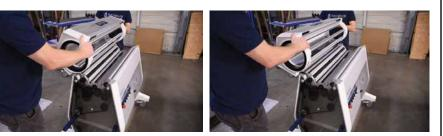
Now, slowly rotate the lid backwards in the opening direction. The lid should lock in the rest of the way.
