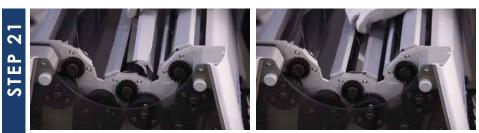
The spacer bar sits on the far side of the helical blade, and the bed knife sits on the near side. Each has a pin on the left side which corresponds to the gear side of the machine.
