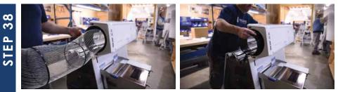
Open the lid and slide the tumbler through, making sure that the plastic fin lines up with the groove.
