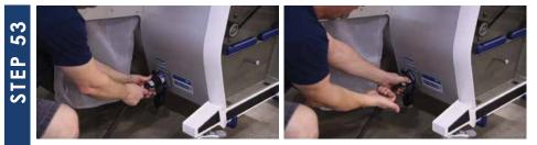
Pull the rubber receptacle cover up. With the Quality Control decal on the power cord facing up, push the plug into the receptacle and rotate it to the right to lock it in place. The machine will power up, the control panel display will indicate errors detected, and the lid will glow red.
