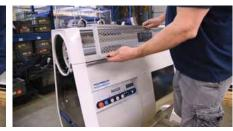
With the lid in the closed position, remove the front screen by pulling the latch on the underside of the lid to the right while pulling the left side of the screen towards you.
