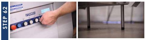
Gravity can be used to increase or decrease the rate at which material moves through the machine by adjusting its tilt angle. Rotate the tilt dial counter clockwise to increase the tilt angle and raise up the infeed side of the machine. The more aggressive the tilt, the faster material will flow. Turn the dial clockwise to lower the tilt angle and reduce the flow rate.
