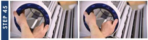
On the outfeed side, lock the tumbler retaining ring by putting your fingers just inside the tumbler, pulling it towards you, and rotating the ring with your thumbs. **An improperly installed tumbler retaining ring can result in operator injury or damage to the tumbler**.
