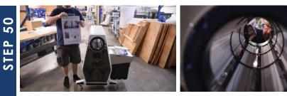
With the lid closed, perform the <u>6-Point Blade Inspection</u>: check to make sure that the space between the tumbler wire and each bed knife is the same. The M108S is ready for safe operation when all blades are fully seated in their channel.
