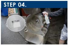
Spritz with a diluted degreasing solution such as warm water and SuperClean.
