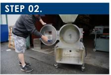
and hit all of these parts and the main body of the machine with compressed air to get rid of as much dust and plant matter as possible.
