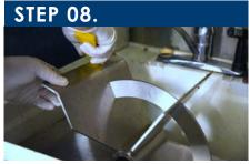
Some material might be caked on the impeller which can be removed with a plastic scraper, and anything remaining can be wiped off. Allow parts to dry before reassembling.
