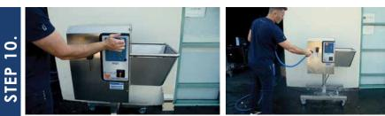
Turn the machine off, unplug it, and rinse it with water.
