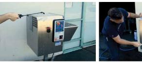
Allow the rollers and chipper to spin while the rest of the machine is sprayed with the cleaner to remove any plant debris and residue. You can use a soft brush to clean off any plant material that is more difficult to remove
