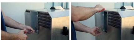
Remove the plexi panel covering the stem chipper on the back side of the machine in the same way.
