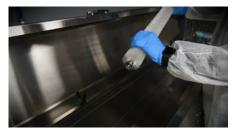
Remove the brush by unclipping it at each end.
