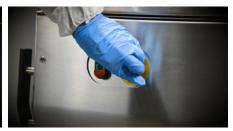
When you push the emergency stop button, you won't be able to press the start button again. This is a safety feature. You'll need to rotate the e-stop to the right to disengage it first, and then push the start button.
