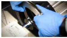
Lift and slide the tumbler frame onto the motor shaft.
