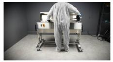
Place the tumbler frame into the washing tub by setting the left side down...
