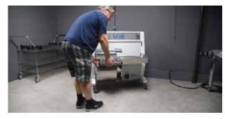
With the window and fascia correctly installed, let's slide the separator into place. There's a rail on the left side of the separator that carries the weight on the left side, but there is nothing carrying the weight on the right side.
