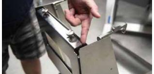
If you notice any gaps, make sure to fix it with the separator out of the trimmer. Do not try to adjust the fascia while the separator is installed in the trimmer.
