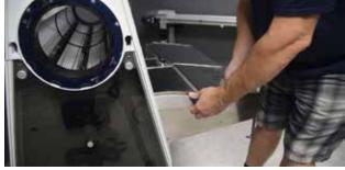
To secure the separator tightly in place, pull the hockey stick all the way up until it is flush with profile of the separator.
