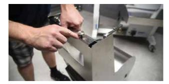
When installing the fascia, be sure to seat it all the way flush to the separator body. The fascia holds the window tight to the separator and seals the vacuum system. You should not have any gaps between the thumb-screw shafts and the fascia cut-outs, or between the fascia and the window.
