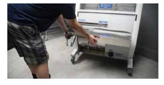
Once you have a couple inches of the rail resting on the left side, lift the right side of the separator up a bit and the separator will slide in easily.
