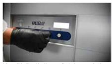
Next, you might want to adjust the machine tilt. That's the switch towards the right of the panel.
