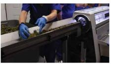
With a single layer of material covering your conveyor belt, set your conveyor speed to a fast setting, say around 80, and turn it on.
