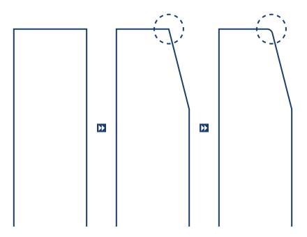
The bedknives on the Mobius are designed as semi-consumables - once the edge begins to 'roll', it's time to swap out that bed knife for a new one. To determine if your bed knife edge has rolled, run the surface of your fingernail at a 45° angle across the blade edge. if the blade edge scrapes the fingernail surface, the edge is still good. if there is no scraping of the fingernail surface, the edge has rolled has rolled has rolled has rolled.
