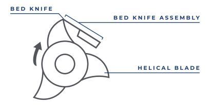
Now that you know how the blades function on the M108S, let's have a closer look at the impact of the shearing action of the two metal surfaces against one another. When you first receive your M108S, the machine and the blades in the machine have been run-in for a minimum of one hour. Any spare blades will not have been run-in. As you operate the M108S for the first few hours, you will notice signs of shearing on the edge of the bed knife. This is normal and expected.
