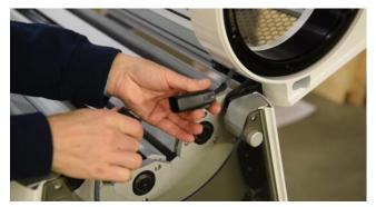
Disconnect the cable that attaches the lid to the M108S body.
