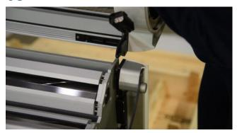
To re-install place the lid hinges so they are sitting on the body hinge.
