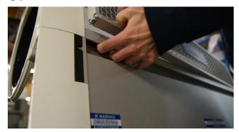
Push the latch and remove the screens on either side of the lid.
