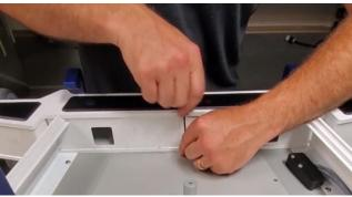
Remove all 6 screws on the electrical box panel to open up access to this area. Next, remove the first and third screw on either side of the control panel and pop it out. You now have access to the electronics and motor on the M108S.
