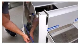
Remove each of the side panels by unscrewing the small silver side panel retainers.
