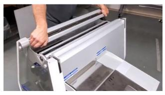
Remove each of the three sets of blade cartridges, placing them in our blade racks (recommended), or somewhere they won't be damaged.
