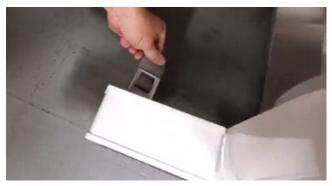
Lock the wheels on the outfeed side of the machine. Place a protective piece of foam on the floor, and add the black sensor override pucks to sensors on each side of the body of the machine. Rotate the handles out, and tip the M108S on its side.
