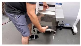
Push down on the 'hockey stick' to disengage the separator; remove the separator and fan housings. If you need further instructions on either of these steps, please see our Separator Removal & Installation Guide.
