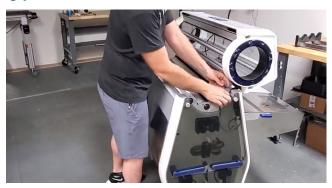
Disconnect the power cord from the machine. Open the lid, disconnect the connection between the lid and the body and remove the lid. For further instruction, see our Lid Removal & Installation video guide.
