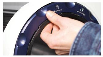
Rotate the retaining ring on the outfeed end clockwise to unlock and then remove it.
