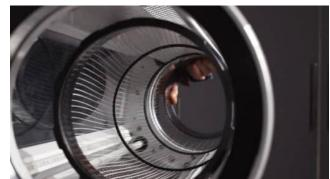
Unlock and remove the other retaining ring. Slide the tumbler out of the lid.
