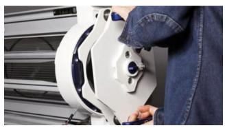
Install the Spring Jack Tool, rotate the handles and valve dial into position and apply enough air to bottom out the Spring Pack.
