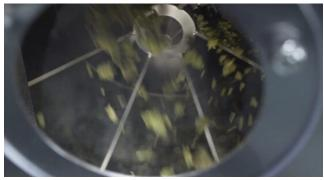
The M210 will mill 35–200 lbs (15–90 kg) per hour, but the last half pound can take up to 5 minutes to work its way through at the end of the run. The coarser the screen, the higher the hourly throughput and vice versa.
