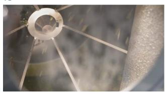
The M210 will mill 35-200 lbs per hour (15-90 kg per hour), but the last half pound can take up to 5 minutes to work its way through at the end of the run. The coarser the screen, the higher the hourly throughput and vice versa.
