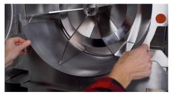
While the perforated screens can be installed in any orientation, the rasp screens are directional. Forward motion of the rotor is clockwise so we want to install the rasp screen with the openings facing to the right.
