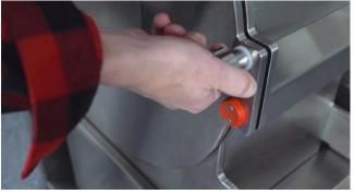
Once the milling screen is in place, close and lock the door. Now we're ready to start milling!
