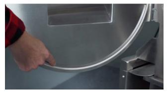
Ensure that the back edge of the screen slots into the groove on the back panel of the chamber which will then align it with the groove on the door.
