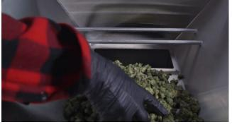
With the rotor running, begin loading plant material into the hopper and sweeping it into the milling chamber. Material can be fed into the chamber as fast as you can sweep it in.
