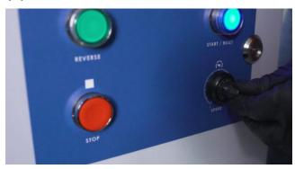
To work through the last half pound, adjust the rotor speed down to 1 or 2 and run for 5-10 minutes. Some strains clear the chamber more easily if the rotor is alternated between forward and reverse every 30 seconds or so.
