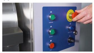
Check the e-stop and, if it's engaged, release it.
