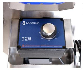
**TIMER** - Turn the timer clockwise to the desired position to energize the motor and rotate the tumbler.
