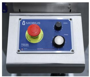
**E-STOP** - Emergency stop button – stops all moving parts on the device.
