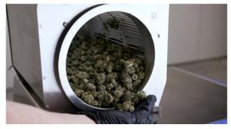
Once the machine is running, it is recommended to check the trim after about 3-5 minutes to make sure the desired trim quality is being achieved with the shearband tension setting. Continue to monitor and check the trim approximately every 5 minutes.
