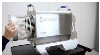
Slide the tumbler through the front plate until the motor hub protrudes through the cutout at the base of the tumbler. Twist the tumbler slightly to latch it on to the motor hub.
