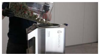
Load with product. Only fill the tumbler about 1/2 to 3 of the way full. Overfilling the tumbler will lead to a lower quality trim and a slower processing time.
