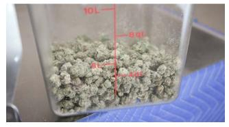
The machine will stop automatically after the chosen time has elapsed. Once the product inside the machine has been trimmed for the specified duration, remove the tumbler end cap and tumbler, and deposit the trimmed product into a container of your choosing.
