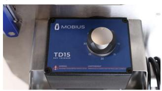
Level the machine back to horizontal using the blue handles and install the tumbler end cap snugly in the front face of the machine. Start the machine by rotating the timer knob to the desired run time.
