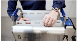
Insert shearband into TD15. Drape the slots in the edges of the shearband over the tabs in the left and right side panels of the machine body.
