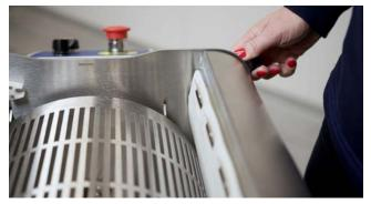
Use the handle on the back of the machine to tension the shearband tight against the tumbler. There is no need to provide additional leverage on the handle, hand tightening is sufficient.
